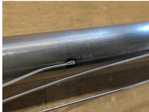
Thermocouple weld mockup
