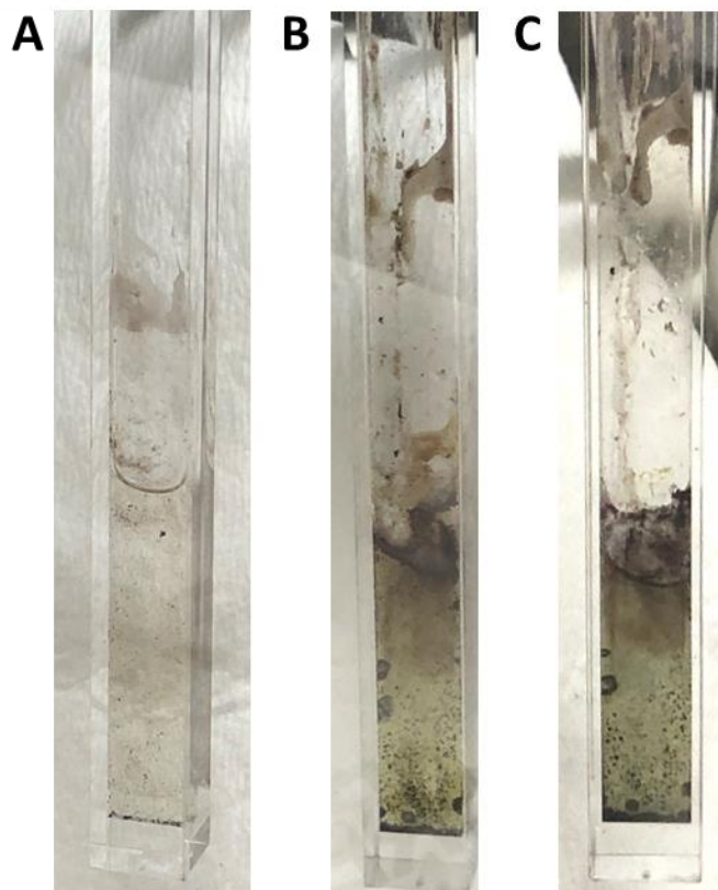
Figure 3-11. Photos of U in LiCl-KCl eutectic at 575°C (a) before the addition of U, (b) after 4 additions of U(IV), and (c) after two subsequent additions of U(III).
