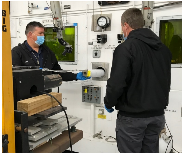
Figure 21: Photograph of insertion of miniHDND in polyethylene insert into the collimator opening at IFEL hot cell.
