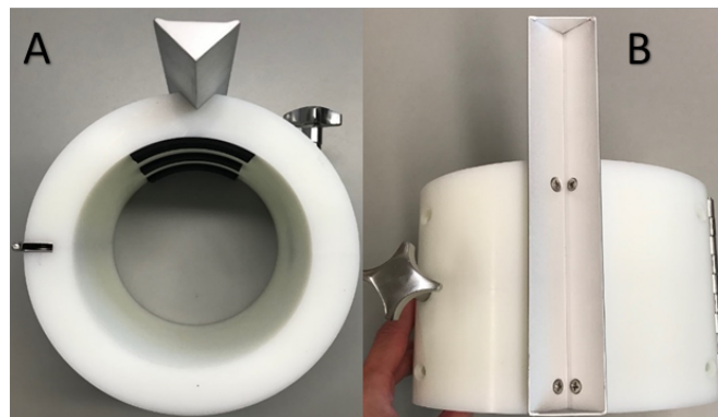
Figure 19: Polyethylene holder with aluminum wedge to hold rod segments; (A) front view and (B) top view.
