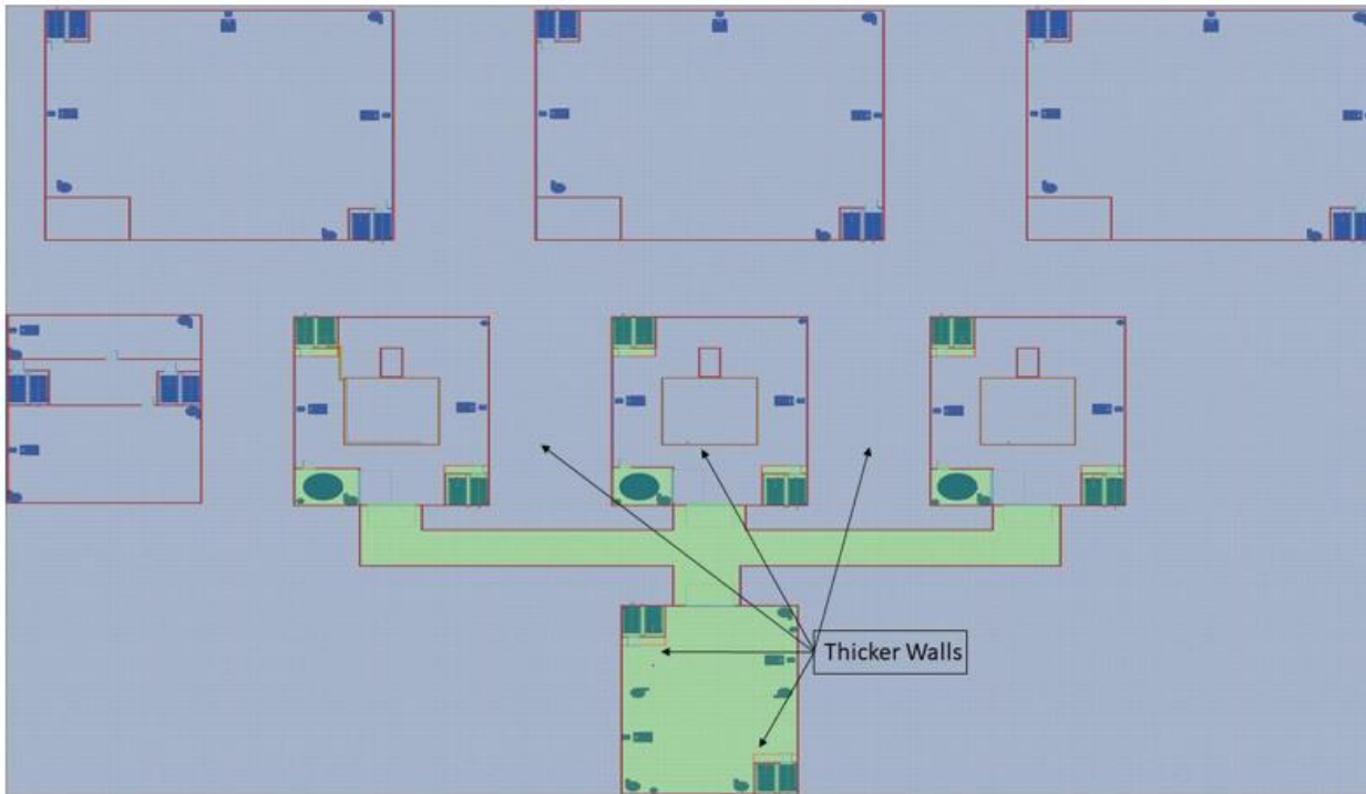
Figure 14 Thicker walls around reactors
