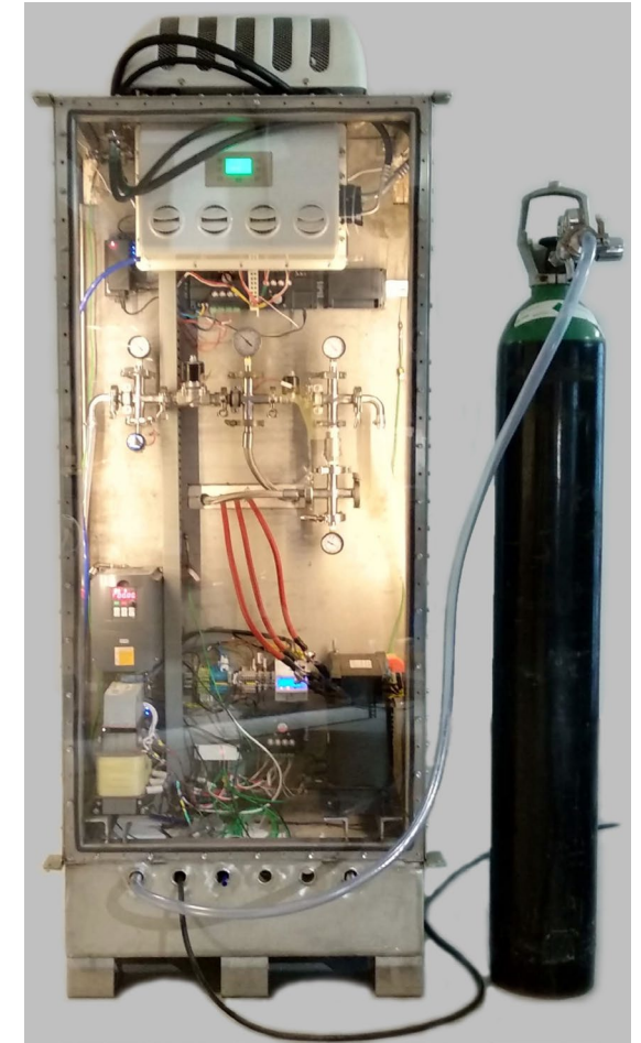
Commercially available forced flow loop from Copenhagen Atomics.
