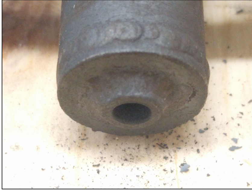
Figure 11. Thermowell (0.125 in. ID) in sodium-filled heat-pipe (0.625 in. OD).
