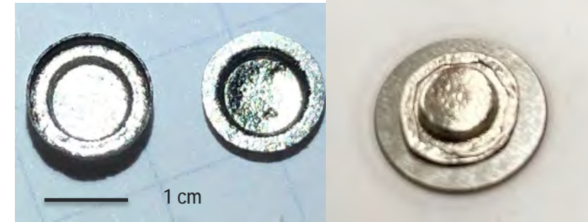
High Temperature Nickel Cells, Open (Left) and Sealed (Right)
