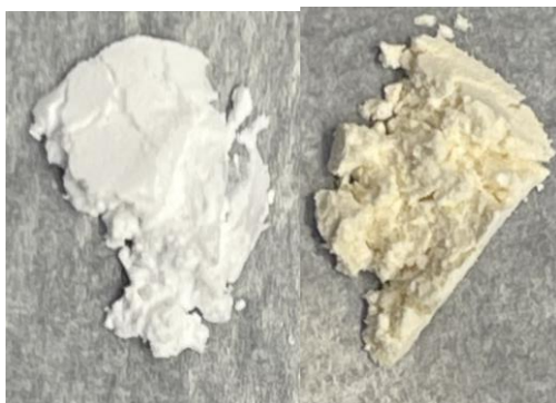
Figure 18: Photographs of pristine CaSDB (left) and CaSDB post 500 Mrad irradiation dose. (right).
