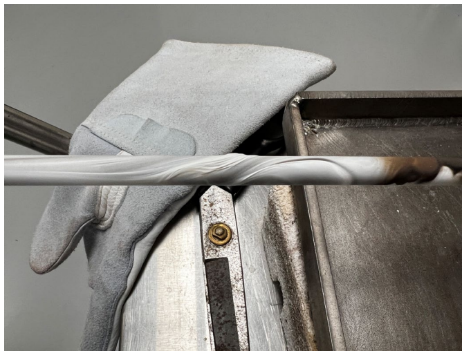
Figure 16. Photograph taken of the cold trap after the initial test run. The white substance is the condensed salt vapor. Length of cold trap tube visible in this photograph is approximately 200 mm.
