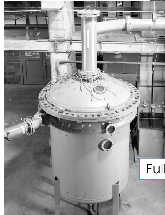
Freeze flange development test rig
