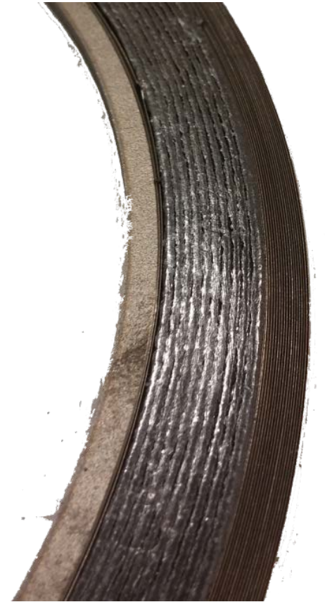
Spiral wound nickel-grafoil gasket
