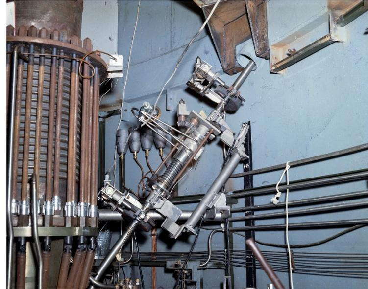
MSRE Sampler-Enricher Mechanism
