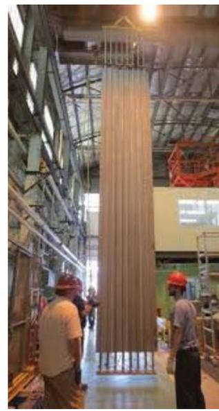
Finned water-cooled riser channels in the NSTF
