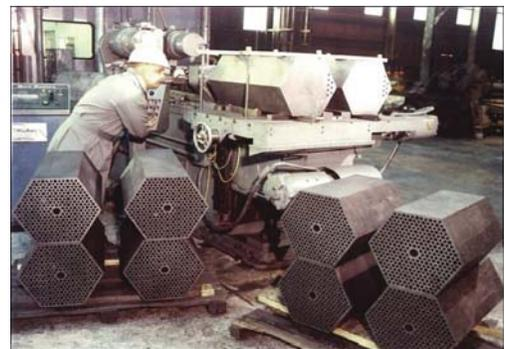
**Gun drilling long holes in Ft. St. Vrain fuel elements
