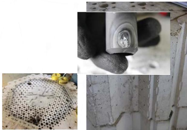
Damaged ceramic core block resulting from block shifting that degraded heater rod electrical continuity causing localized hot spots - 4 need to be replaced
