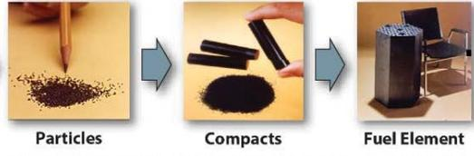
TRISO-coated fuel particles (left) are formed into fuel compacts (center) and inserted into graphite fuel elements (right) for the prismatic reactor
