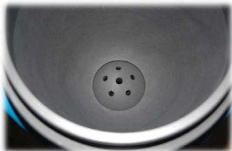
Coater converging section and gas nozzle
