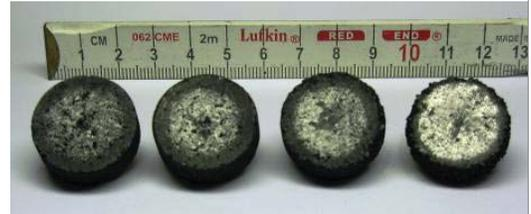
Oxidation/Degradation of graphite samples
