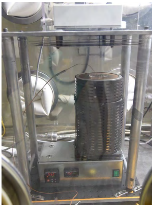
Figure 3. Experimental density setup showing bottom-loading balance on the stand above a furnace with quartz lid and thermocouple inserted inside the AFCI glovebox.
