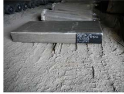
Alloy 709 plates fabricated from 45,000 lb commercial heat
