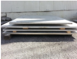
Alloy 709 plates fabricated from 45,000 lb commercial heat
