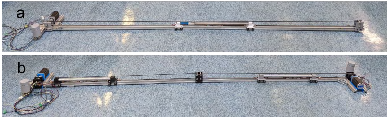
Figure 8: Hardware fabrication a) detector moving system; b) dual control rods moving system.
