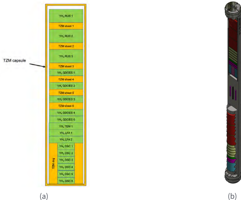
Figure 8-3: Schematic of specimen stacking in TZM capsule. (a) A 2D cross section of the TZM irradiation capsule. Green: yttrium dihydride samples; orange: TZM fixturing. Samples are labeled with intended PIE technique. (b) A 3D rendering of two TZM capsules intended for a single temperature.
