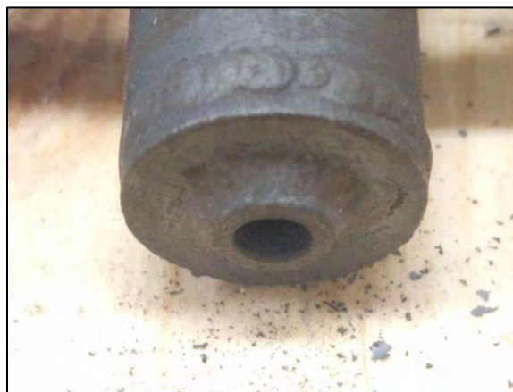
Figure 2. Heat Pipe centerline thermocouple measurement points
