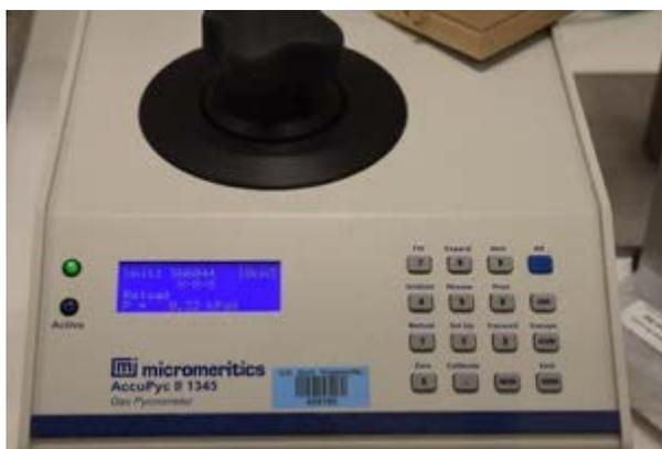
Figure 6. Micromeritics AccuPyc II 1345 gas displacement pycnometer
