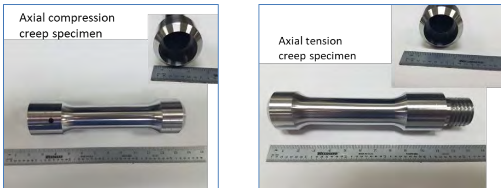
Fig. 18. Gr. 91 specimens for multi-axial stress creep testing.
