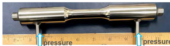
Fig. 14. Picture of the SBSMT specimen for evaluation of primary load effect
