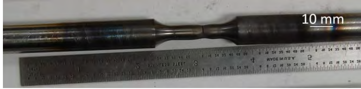
Fig. 17. Photograph of the failed TB03 specimen.
