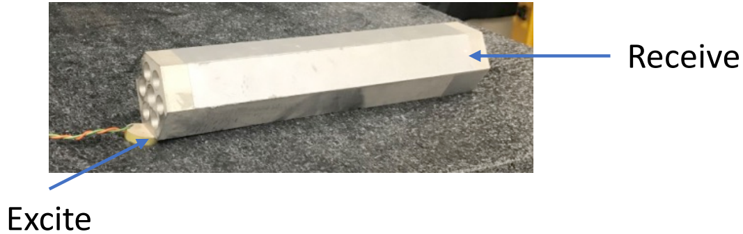
Figure 4: Experimental setup used to demonstrate the ability of RUS to detect small changes in a system.
