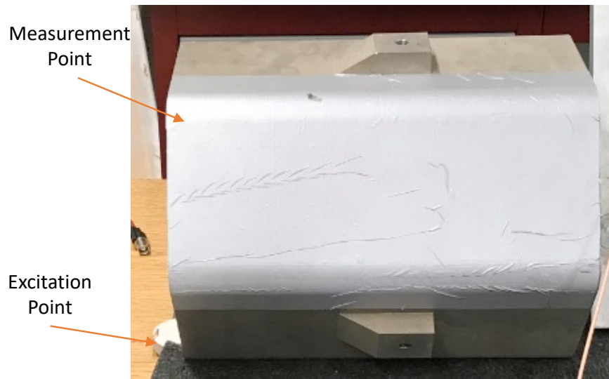
Figure 1: Experimental setup for evaluating the feasibility of using ambient noise for RUS measurements.
