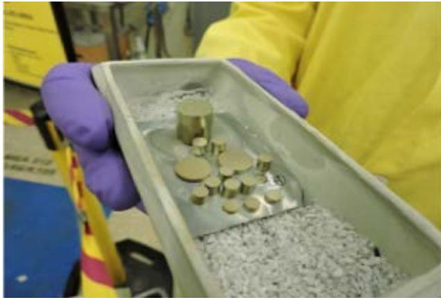
Figure 3. 40%U-ZrH<sub>x</sub> pellets fabricated by powder metallurgy. Samples were fabricated in dimensions required for thermophysical property measurements.
