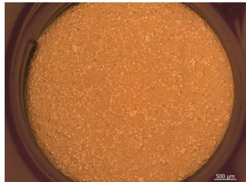
Figure 4. Bright field optical image of an as-fabricated 40%U-ZrH<sub>x</sub> pellet cross-section.
