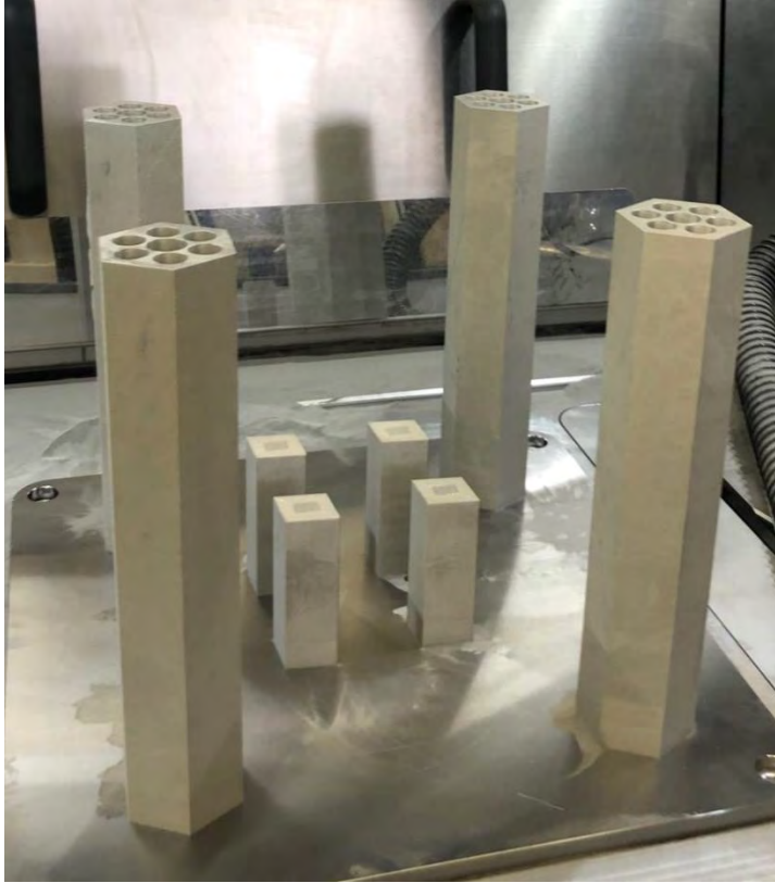
Figure 6. Four 11" tall sections of the Block 7 design within the build chamber of an EOS M400-4. Center blocks are to be used for mechanical testing.
