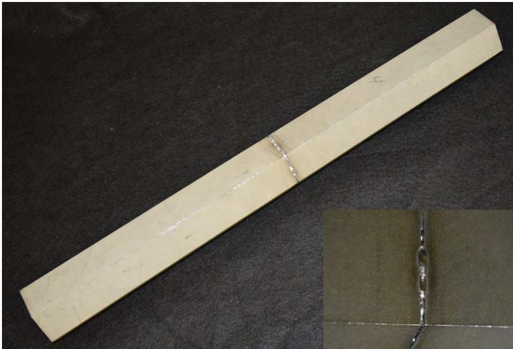
Figure 9. Image showing completed 22" long Block 7 design with a single tier weld performed during a rotary butt weld in an electron beam welder. Inset shows surface quality of the weld. Imperfections in fill at the corners as seen in the inset can be easily remedied with a cover pass.
