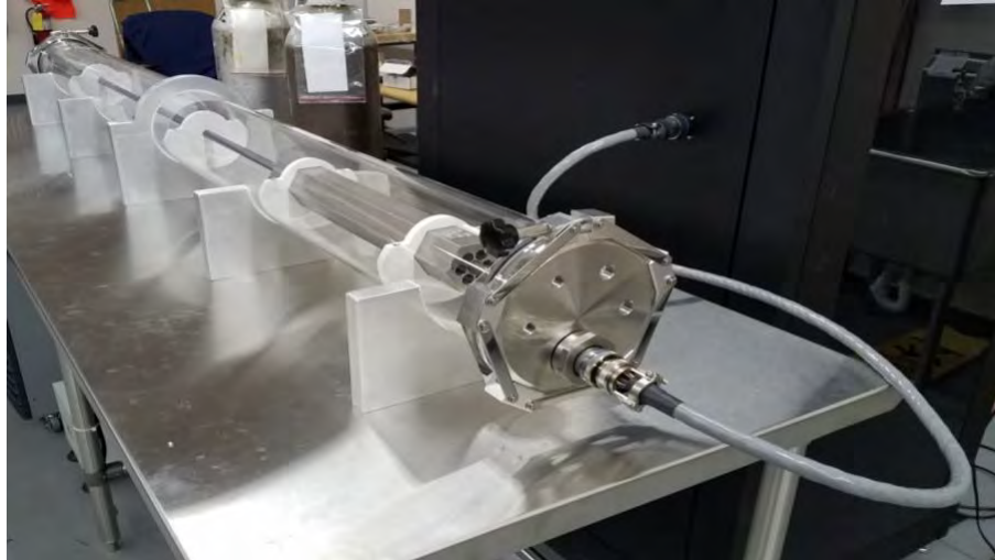
Figure 4: SPHERE test bed and seven-hole test article.
