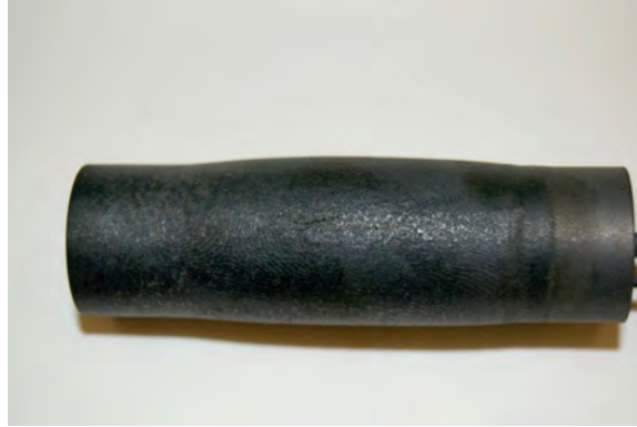
Figure 1.2: Typical pressurized creep specimen tested to a failure. The thin-walled capped tube is pressurized which induces a biaxial stress state in tubular shell. The principal stresses are, approximately, \sigma_1 = 2\sigma_2 with \sigma_3 = 0 . Figure reproduced from [52].
