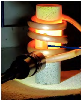
Induction heating setup
