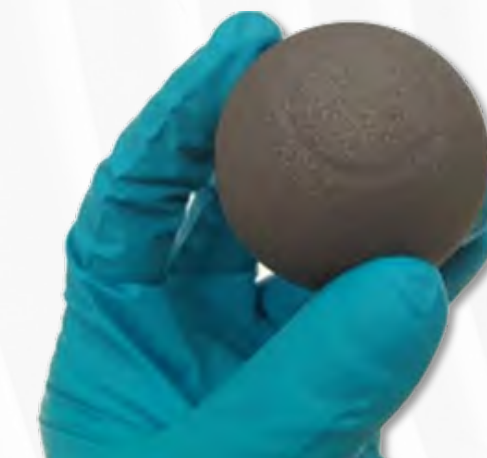
First fuel form pebbles produced at ORNL, Fall 2016
