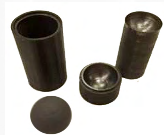
Prototype pebble mold
