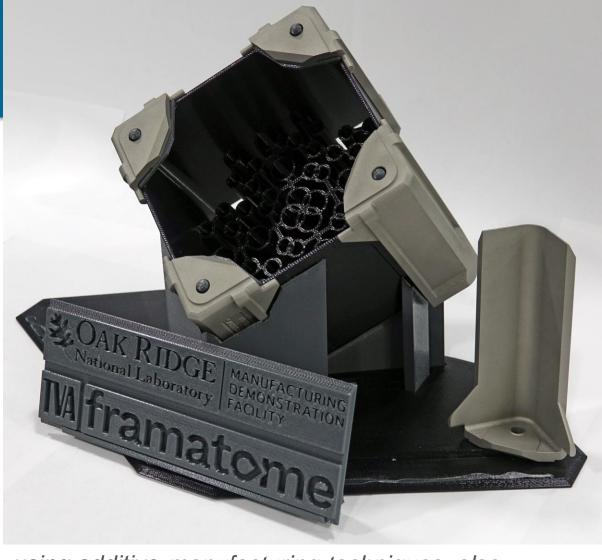
"The fuel assembly channel fasteners were printed at ORNL using additive-manufacturing techniques, also known as 3D printing, as part of the lab's Transformational Challenge Reactor Program and installed on ATRIUM 10XM fuel assemblies at Framatome's nuclear fuel manufacturing facility in Richland, Washington."
