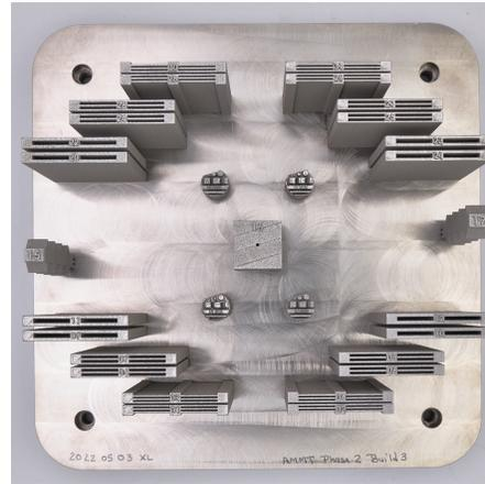
Build 2.1 - designed to capture tensile property trends at **taller build heights and** acquire examples of **intermediate** UTS and YTS values
