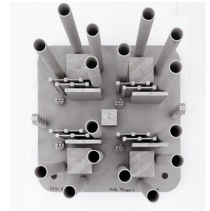
Build 1.1 – designed to capture **baseline data** i.e., thermal history based on part geometry and laser module used to fuse the material
