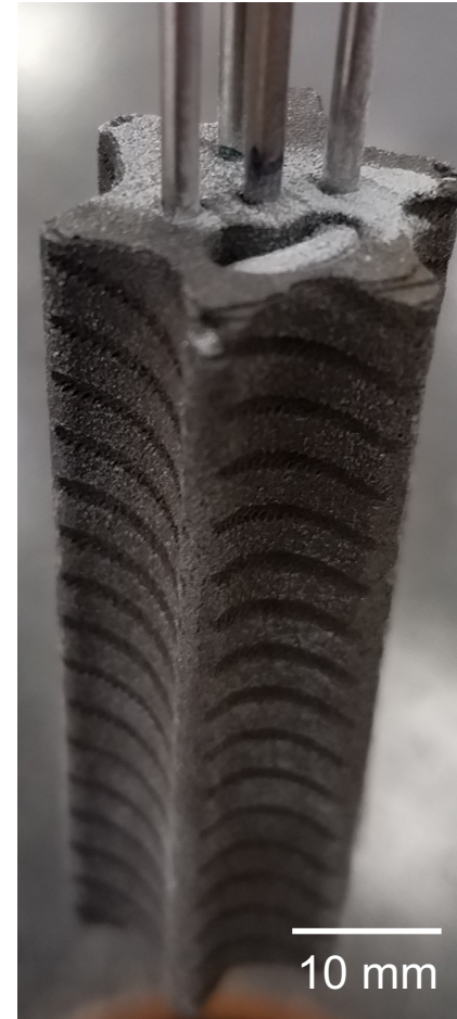
Option 2: Print part with void region to be filled with sensor, other materials (e.g., fuel), and loose SiC powder
