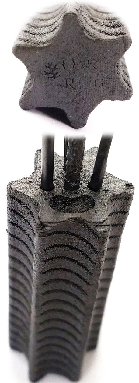
Both: Densify entire assembly using CVI, embedding sensors in dense SiC part
