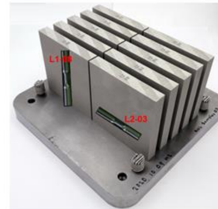
Specimens machined from plates of ORNL Build 20201009M2 in two build orientations: Horizontal vs vertical.
