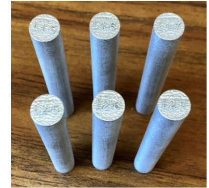
Specimens machined from rods of ORNL Build 20190315M2.
