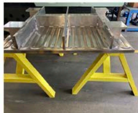
Chamber endwall in fabrication at Kurt Lesker showing hydro-cooling channels
