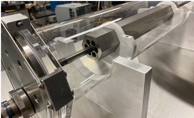
Quartz tube allows tests in vacuum or inert gas environments
