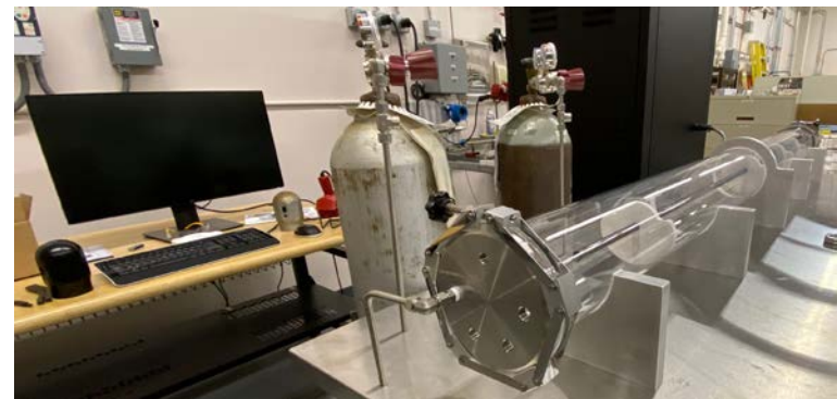
Test stand gas/vacuum/cooling end and control computer
