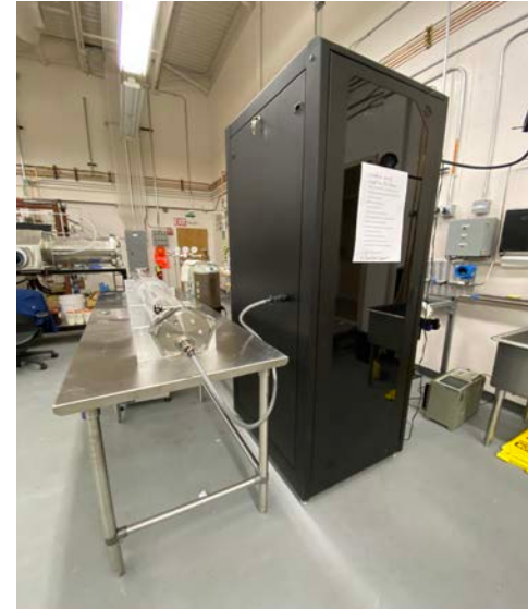
Test stand and power and instrumentation cabinet
