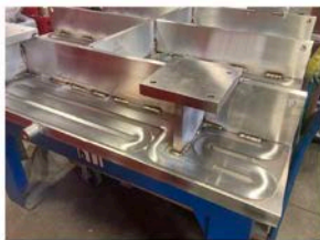
Chamber bottom with supports and hydro-cooling channels
