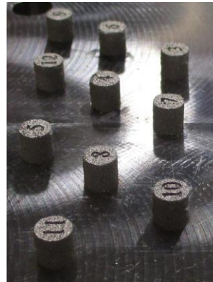
Nb1Zr build printed on the EOS M400 machine at LANL.
