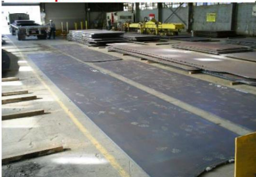
Photograph of 1 st commercial heat A709 plates in as-rolled condition
