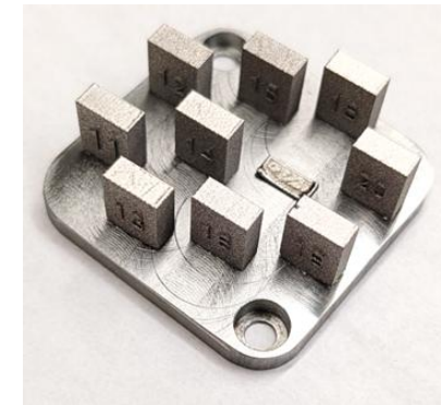
Printed Nb-1Zr cubes on Mo build plate at ORNL.
