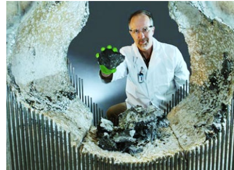
LWR Melt Coolability and Concrete Interactions (MCCI) Facility for severe accident experiments
