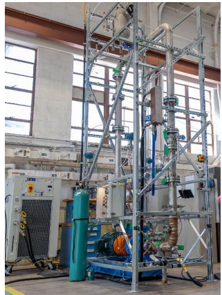
Pressure drop Experimental Loop for Investigations of Core Assemblies in advanced Nuclear (PELICAN)
