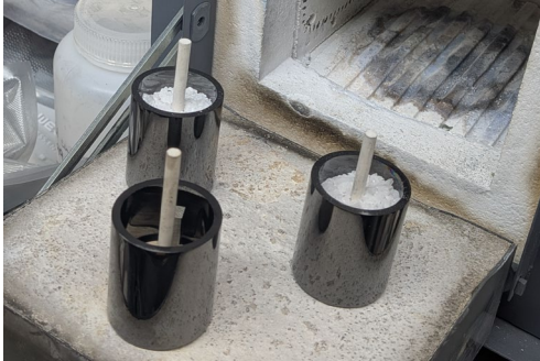
Wrought SS316 exposure complete w/ Terrapower and as-purchased salt
