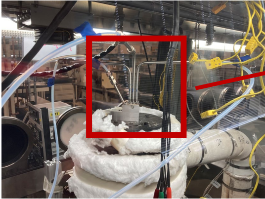
Modified triple bubbler installed in the molten salt flow loop
