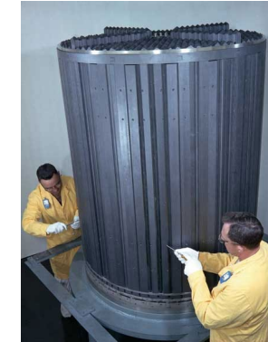
MSRE core (left and center) and graphite block arrangement (right) [1]
