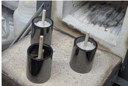
Crucible setup - static immersion in molten chloride salt
