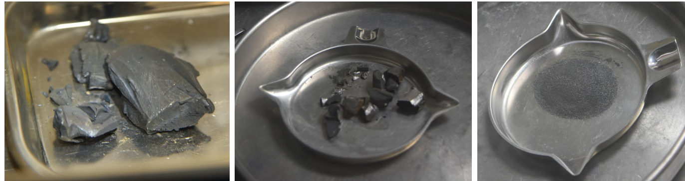
Pu-Am metal material, ~350g (left), ~100g Pu-Am metal starting material (middle), Pu-Am powder after hydride/de-hydride (right)
