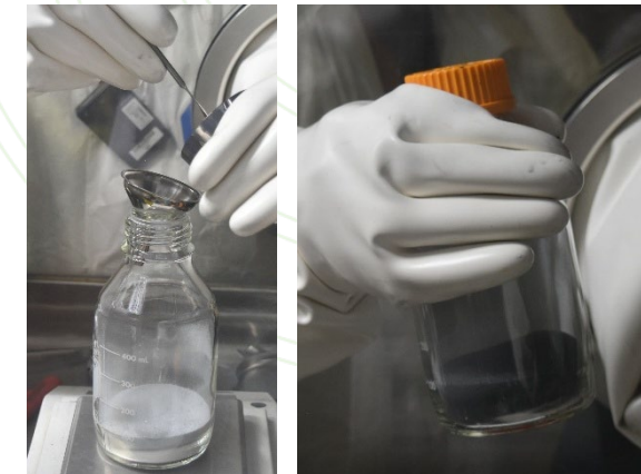
NaCl and \text{NH}_4\text{Cl} in mixing container with fractions of Pu-Am metal being added (left) and NaCl, \text{NH}_4\text{Cl} , and Pu-Am metal mixed
