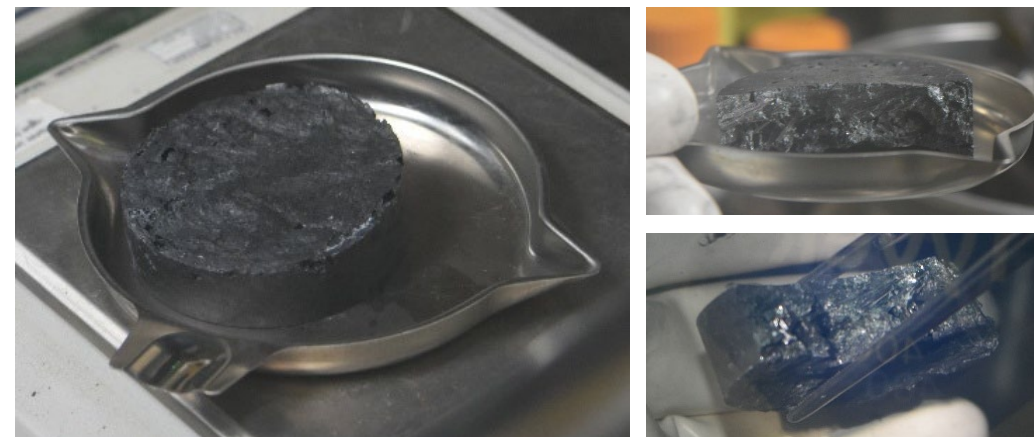
40\text{PuCl}_3\text{-}9\text{AmCl}_3\text{-}50\text{NaCl} (target) fuel salt puck (left) and broken up puck (right)
