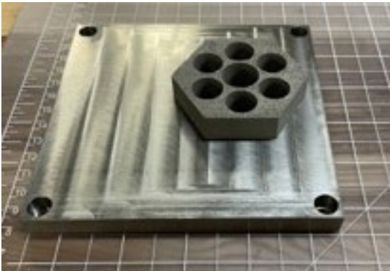
Seven-hole core block sample fabricated from TZM alloy at LANL.
