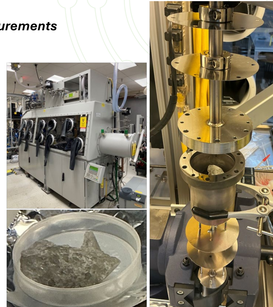
Top Left: Newly commissioned TGAP (Tritium Gas Absorption Permeation) glovebox. Bottom Left: FLiBe ( \text{LiF-BeF}_2 ) salt used in the first tritium solubility measurements. Right: TGAP permeation test section loaded with 43.25 g of FLiBe.
