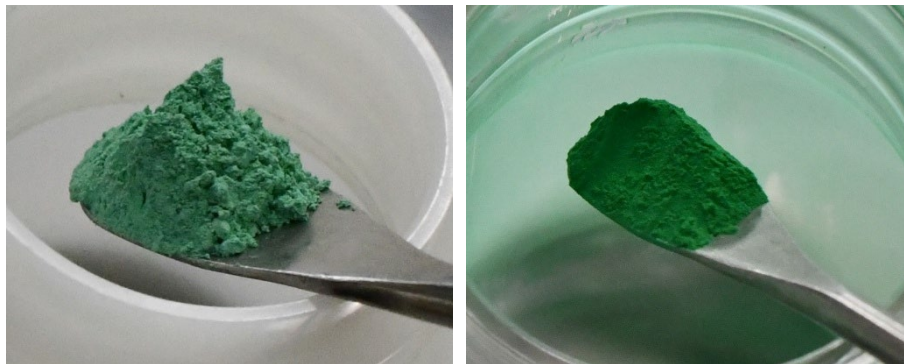
As purchased \text{UF}_4 with oxide impurities (left), purified \text{UF}_4 (right)
