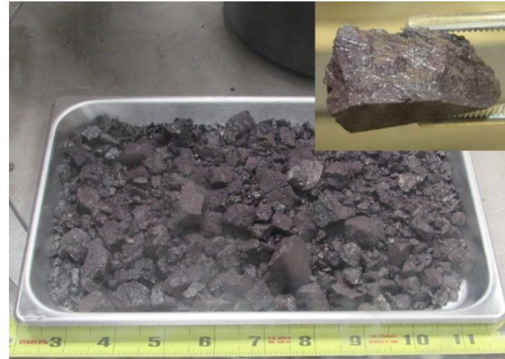
\text{LiCl-KCl-UCl}_3 (43.4 wt% \text{UCl}_3 ) salt produced by \text{ZnCl}_2 chlorination.
