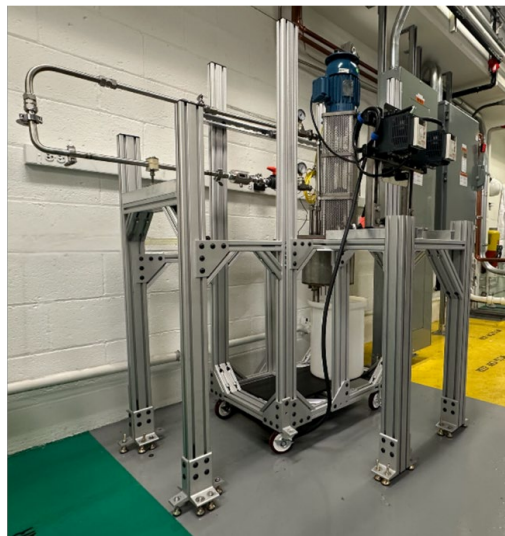
Photo of water test loop
