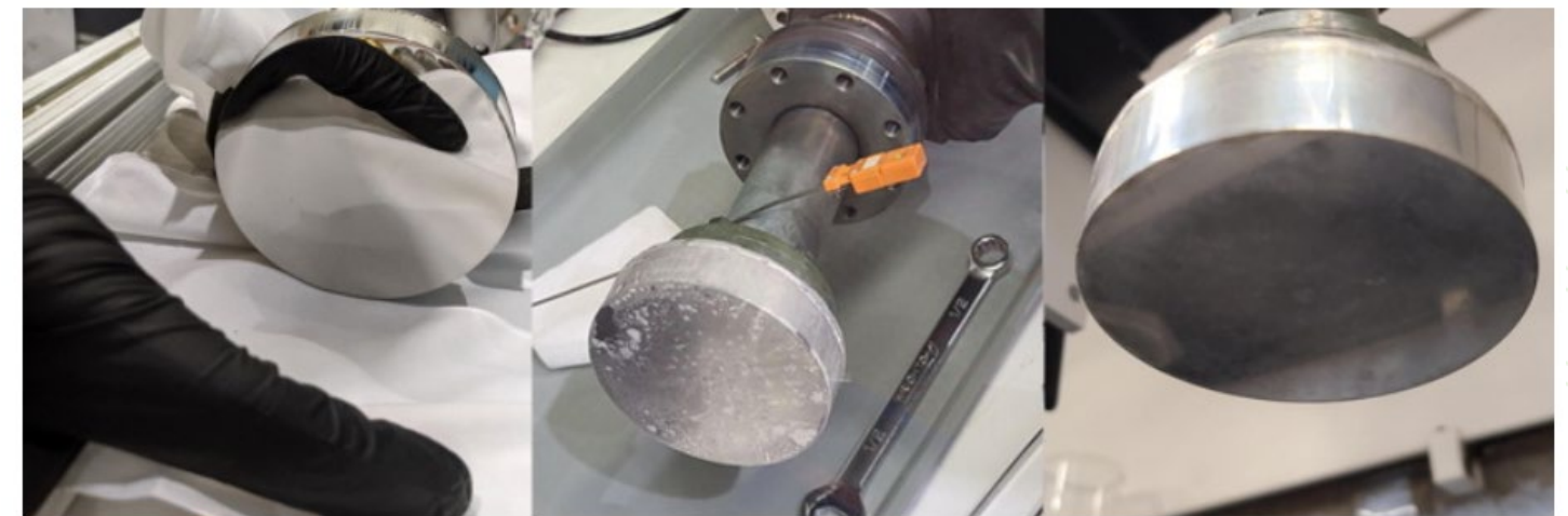
Fig. 6. The bottom surface of the heater cell before testing (left), directly after testing (middle), and after cleaning in an ultrasonic water bath (right).
