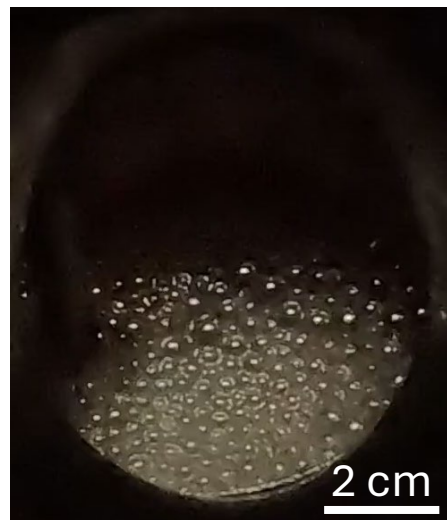
Sparging salt at 0.2 L min -1
