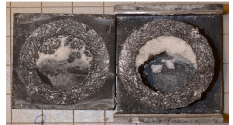
Dendrite growth on mica and graphite rings compressed between Inconel 625
