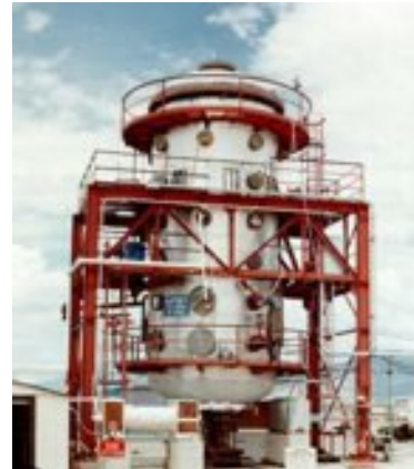
The 185-foot Drop Tower Facility provides a controlled environment for testing small and large test items.
