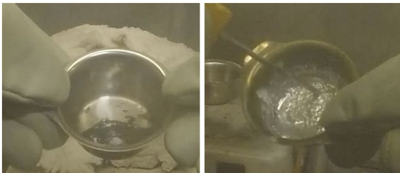
Figure 1 NaK control before heating (left) and after heating (right)
