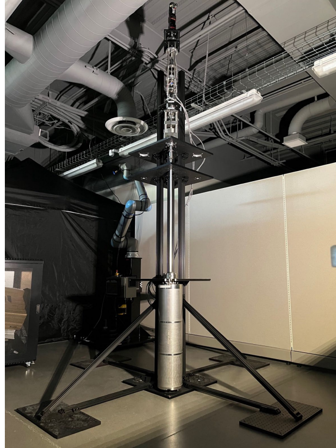
Start of RCS assembly in qualification stand at ESRL
