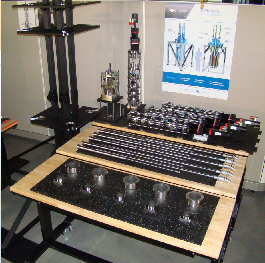
Final fabricated parts for the MARVEL RCS
