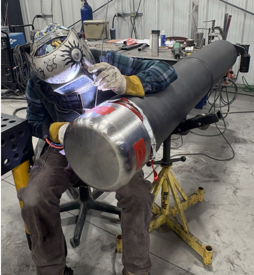
Reactor upper plenum and core barrel getting welded
