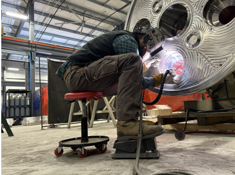
Reactor upper plenum and core barrel getting welded
