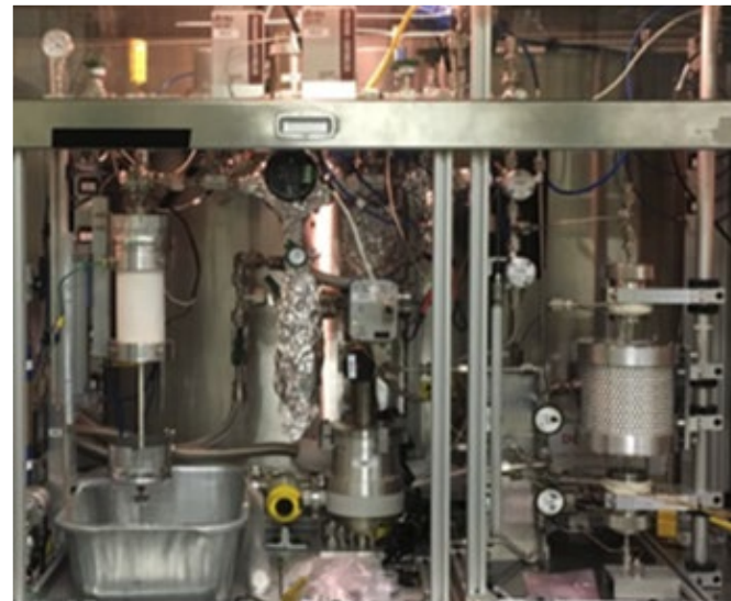
SGAP test section with MgO single crystal sample (it's transparent!)
